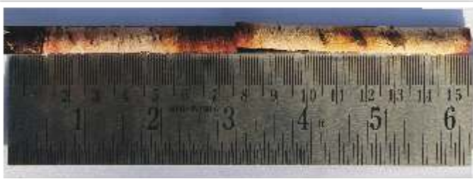
Increment core showing poor heartwood formation (18 year old tree growing on fertile agriculture soils)
