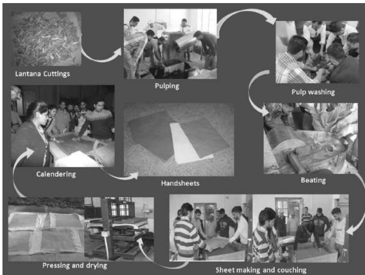
Fig. 40. Steps of making handmade paper from Lantana camara
