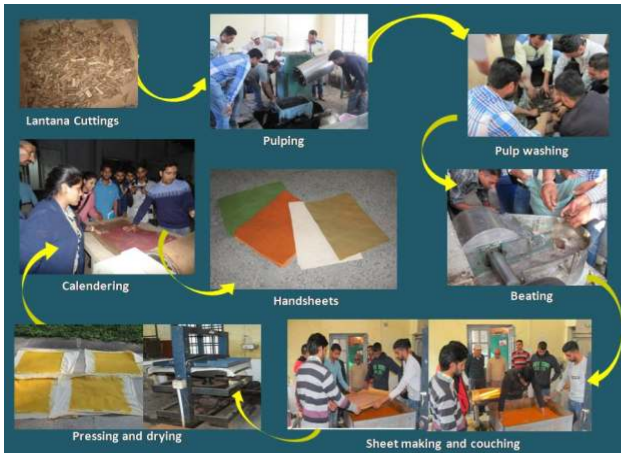
Steps of making handmade paper from Lantana camara
