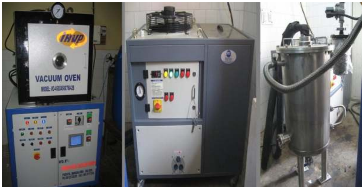
Microprocessor controlled vacuum chamber for heat treatment of wood
