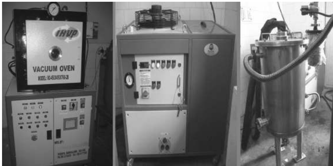
Vacuum oven Condenser & filterChilling unit
